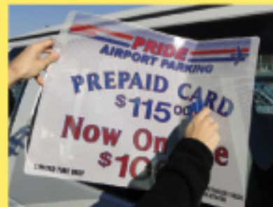
STEP 11. Gently squeegee down the rest of the graphic.
