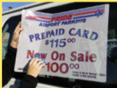
STEP 12. Gently squeegee down the rest of the graphic.
