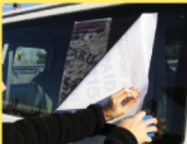
STEP 10. Remove remaining liner and discard. Make sure not to let graphic stick to its self.
