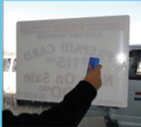
STEP 7. Squeegee out all remaining water from the center out, keep spraying with water while doing so to keep it lubricated.
